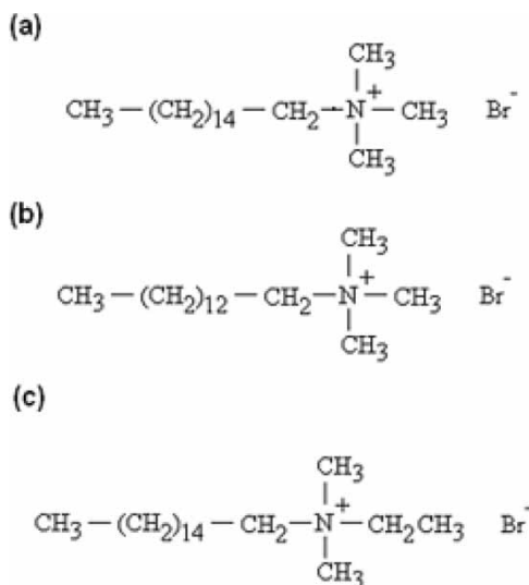
Figure 1. Molecular structures of (a) cetyltrimethylammonium bromide (CTAB), (b) trimethyltetradecylammonium bromide (TTAB), and (c) ethylhexadecyldimethylammonium bromide (EDAB).
